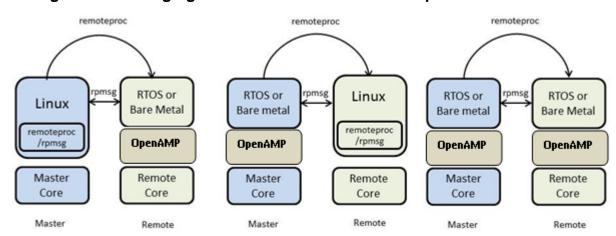
Figure 1-1. Managing Remote Processes with the OpenAMP framework
