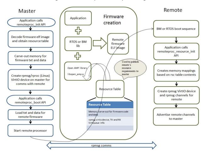
Figure 3-1. remoteproc Conceptual Diagram
