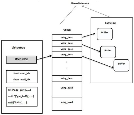
Figure A-2. The Virtqueue and Vring
